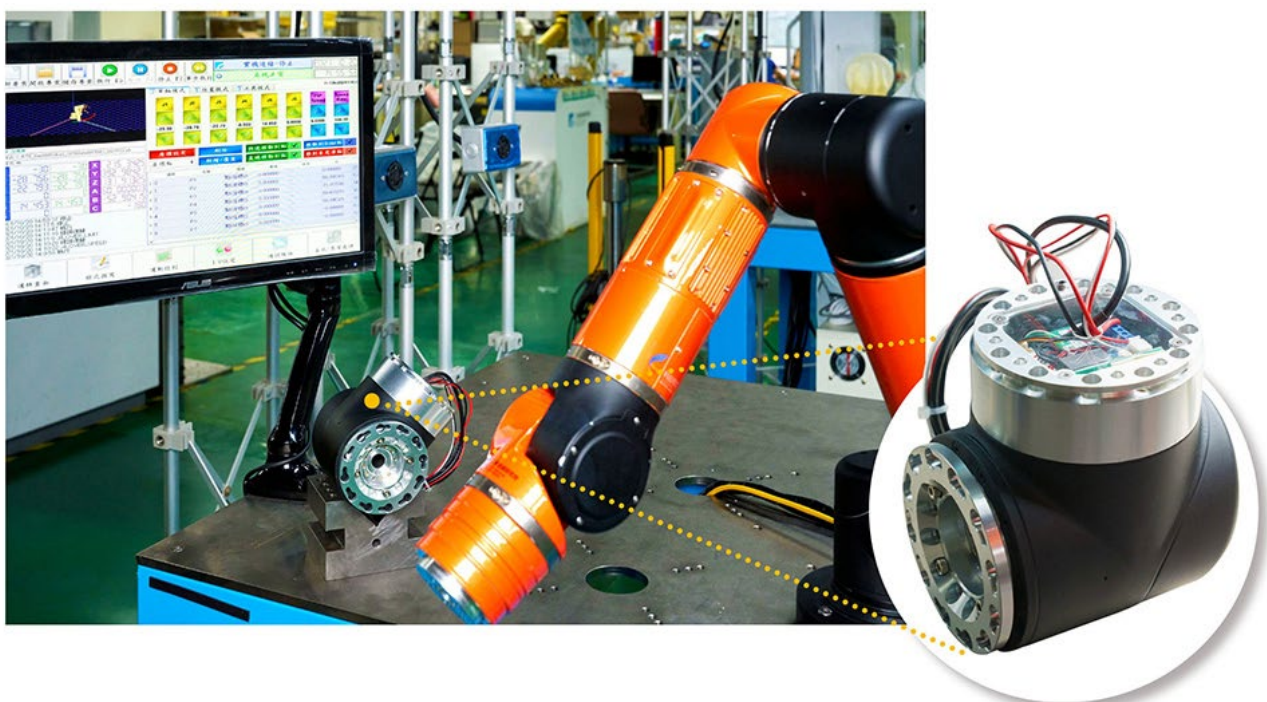
ITRI's Software-defined Augmented Robot Joint allows for modular designs, and has the
